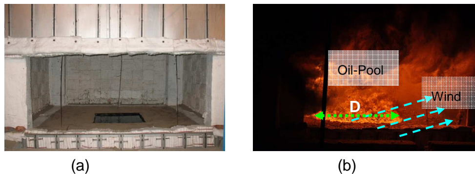
Figure 6-10 (a) Test setup for realistic compartment fire (b) Attainment of flashover in fire test [117]
