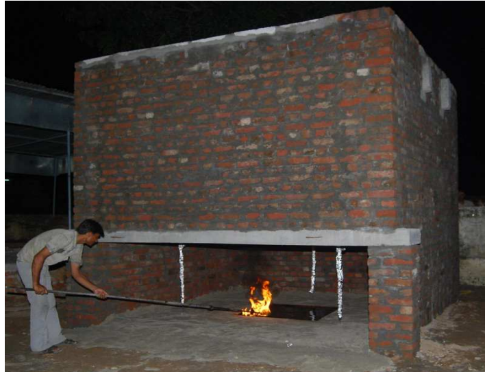
Figure 6-1 Set-up of a brick masonry with a pool fire for test [Reproduced from 120]
