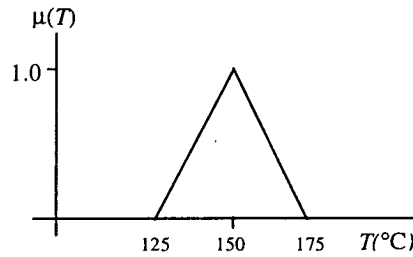
Fig.2-3 Fuzzy set of “temperature is about 150 °C”
