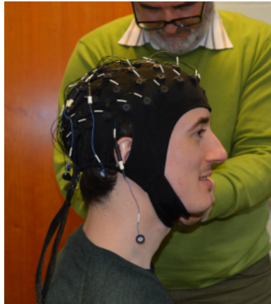
Figure 2.2: Picture of an EEG cap worn by a man seated in front of a computer. Courtesy of Dr. Mario A. Parra, Psychology Department, Heriot-Watt University.
