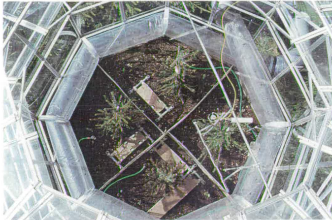
Figure 2: View through the top of a chamber, showing barriers and removable walkways
