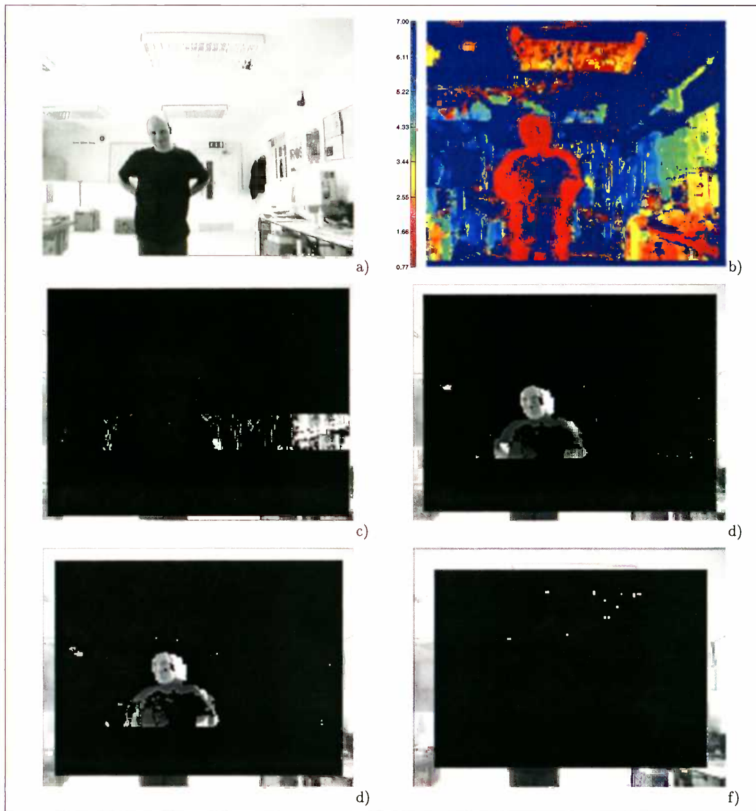
Figure 5.8: Constrained search space using both depth and geometric information (general case): images (a) and (b) show the grey -level and depth information of the scene while images (c)-(f) show respectively the levels 0, 4, 5, and 8 of the image pyramid where the blacked-out areas corresponds to the elements eliminated from the search space; the camera's tilt angle is 10^\circ above the ground plane.
