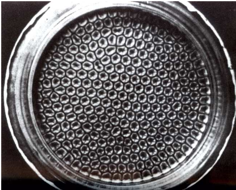
Figure 2.3: The spontaneous emergence of pattern in the Bénard cell convection experiment (from Kondepudi and Prigogine, 1998. No scale is given with the original reference).
