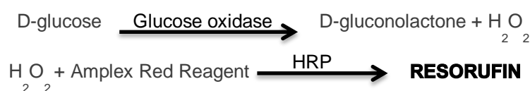
Figure 2.2: Principle of coupled enzymatic reactions used for the detection of glucose [403].
