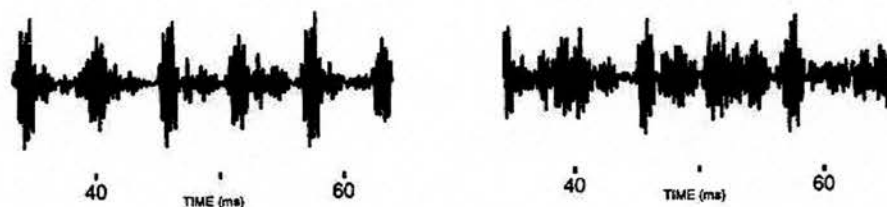
Figure 3.6: The waveforms of synthetic tokens used for noise ratings by Hanson (1995), generated by using a bandpass-filter (center: 3\text{kHz} , bandwidth: 600\text{Hz} ). The waveform of a token (left) with periodic component of moderate spectral tilt and aspiration noise. The waveform of the token (right) shows a token with larger spectral tilt in the source and aspiration noise. (from Hanson, 1995)
