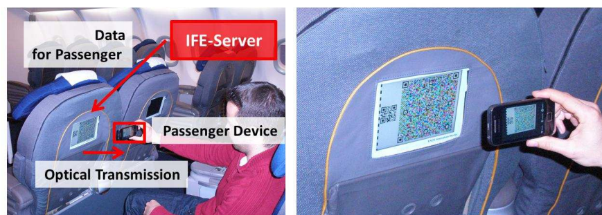
Fig. 1. Left: Setup for the transmission of passenger specific data from the central IFE server to the mobile device. Right: Typical distance between mobile device and display.
