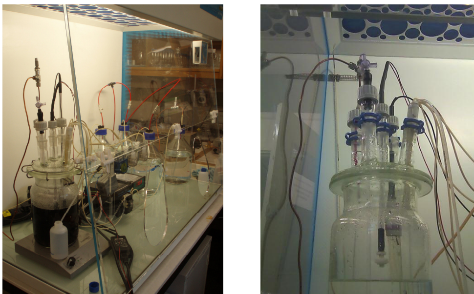
Figure 7.1: A: Overview on the chemostatic reaction vessel. The black colour of the reaction reflects the presence of mackinawite in the system. B: Zoom on the pH electrode and the float controlling the constant volume of solution in the chemostat.
