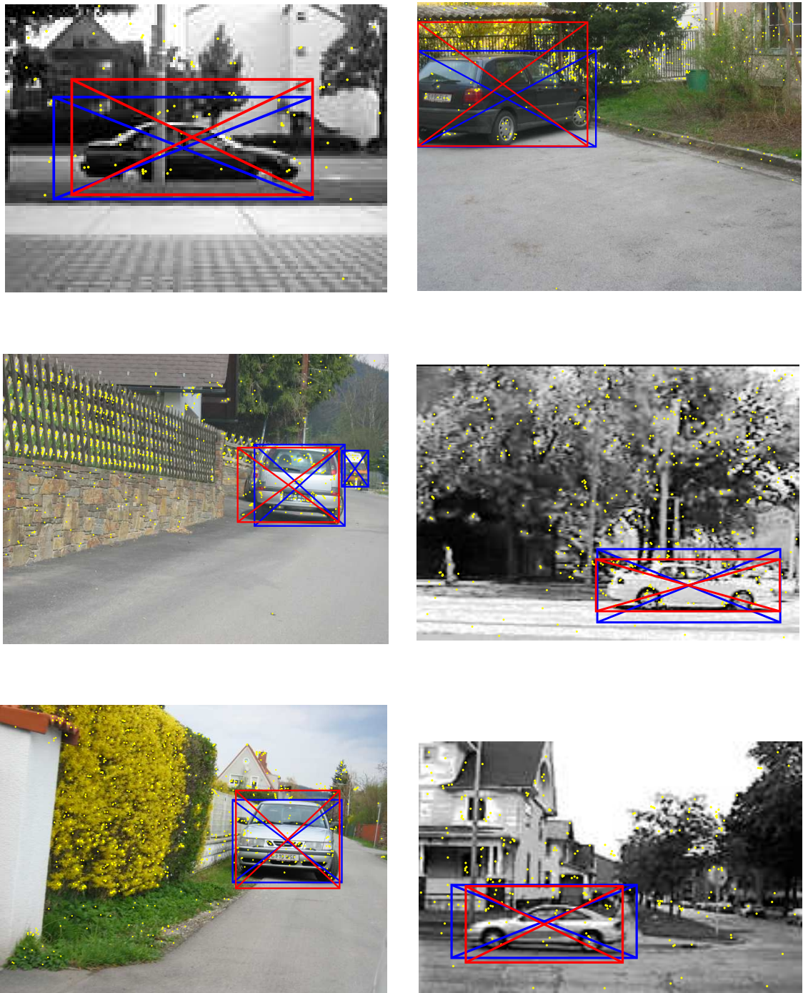
Figure 6.26: Lowest-confidence images with correct detections for car classifier for GTF as in Table 6.8.
