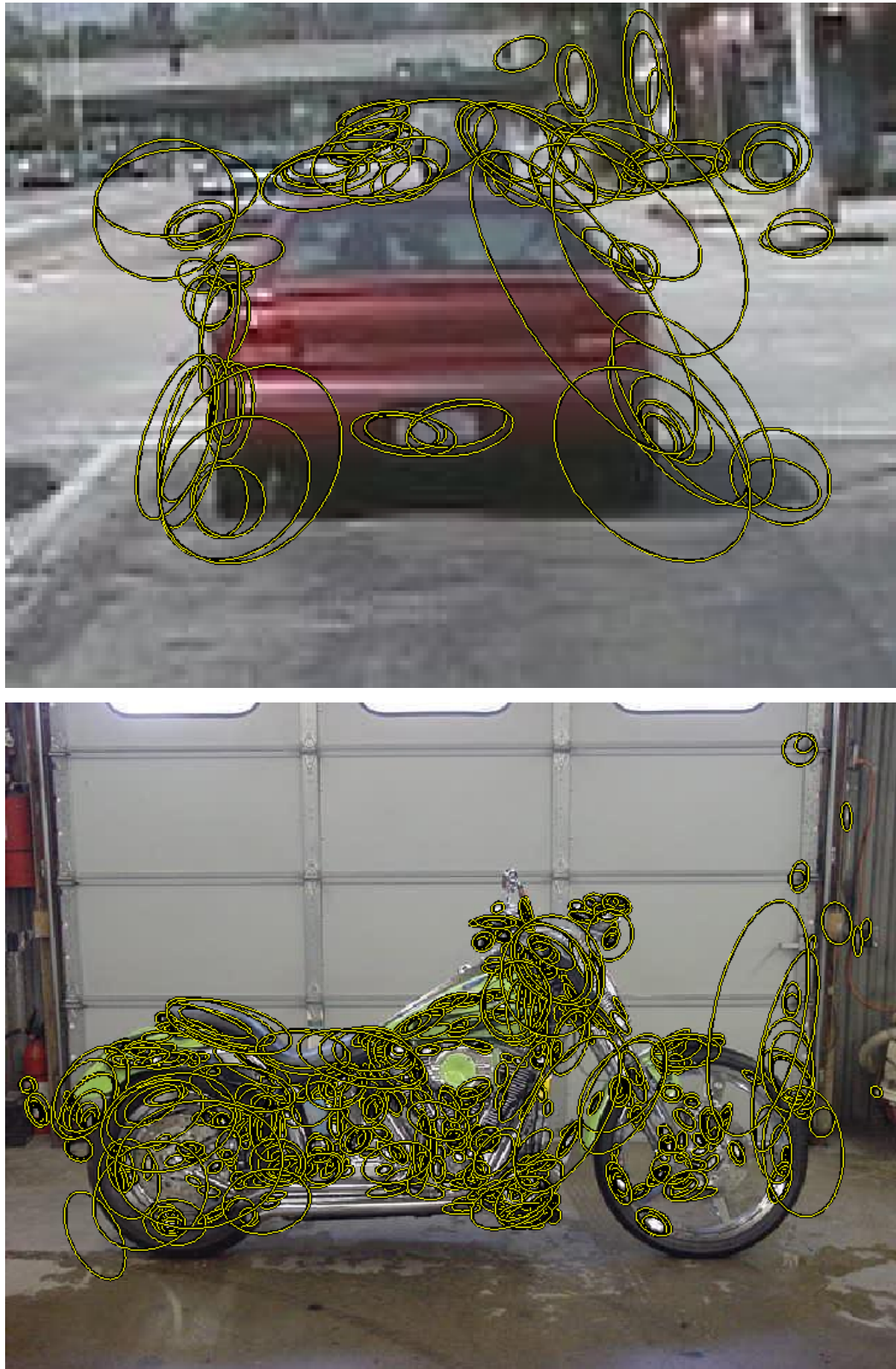
Figure 2.1: Regions of interest found by the Harris affine detector in two sample images.
