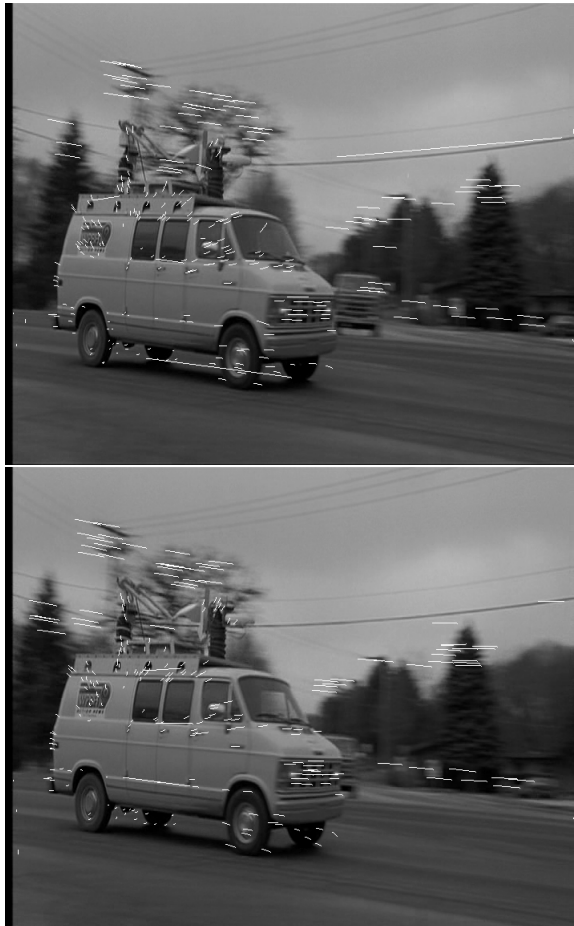
Figure 4.2: Features matched between frames 46 and 47, and frames 47 and 48 of Groundhog Day sequence: lines show the motion of a feature between consecutive frames.
