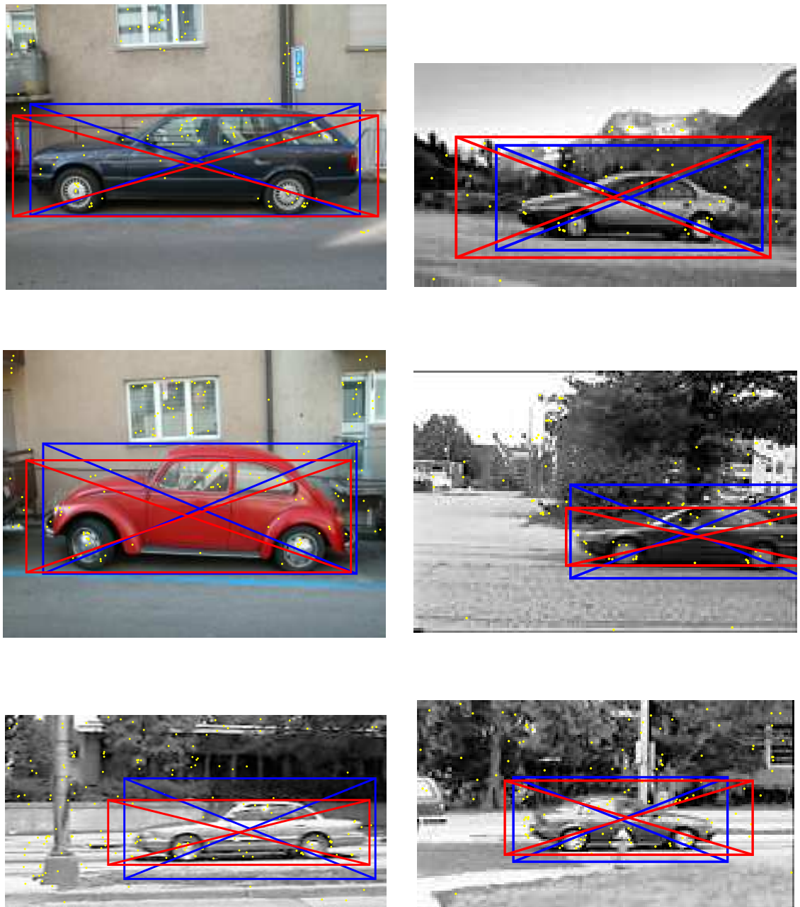
Figure 6.22: Highest-confidence images with correct detections for car classifier for GTF as in Table 6.8.
