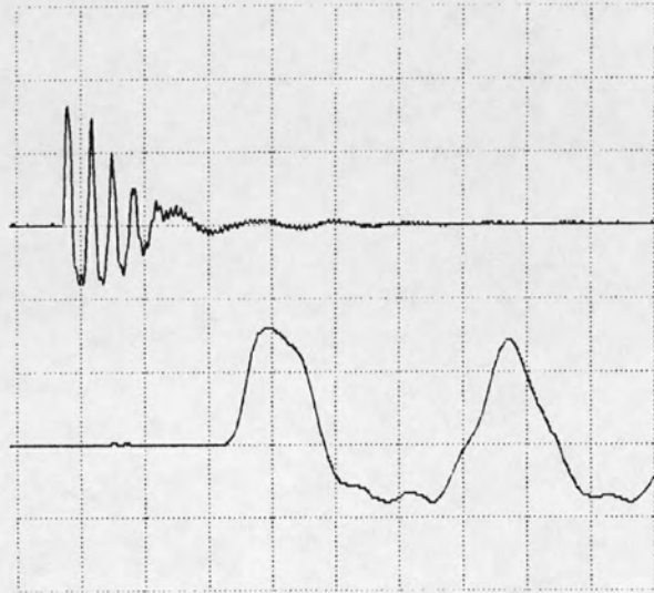
Fig.4.6.d. Screen dump of plastic/plastic collision. Upper trace: Resiliently mounted anvil/plastic hammer. Lower trace: Upper trace with 10x expanded timescale.
