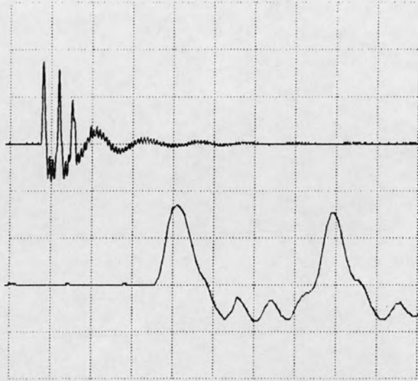
Fig.4.6.c. Screen dump of plastic/steel collision. Upper trace: Resiliently mounted anvil/steel hammer. Lower trace: Upper trace with 10x expanded timescale.
