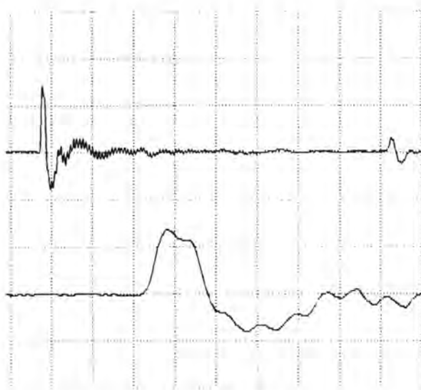
Fig.4.7.b. Screen dump, resiliently mounted anvil. Upper trace: Flat enamel anvil and cusp hammer. Lower trace: Upper trace with 10x expanded timescale.
