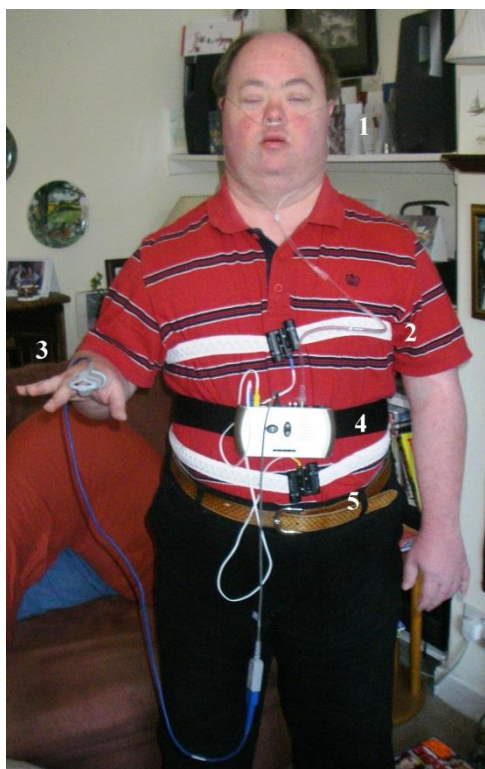
Figure 19: The Embletta ® Gold ™ equipment in situ: 1) nasal pressure cannula; 2) thoracic effort band; 3) pulse oximeter; 4) main unit, including body position sensor; 5) abdominal effort band.
