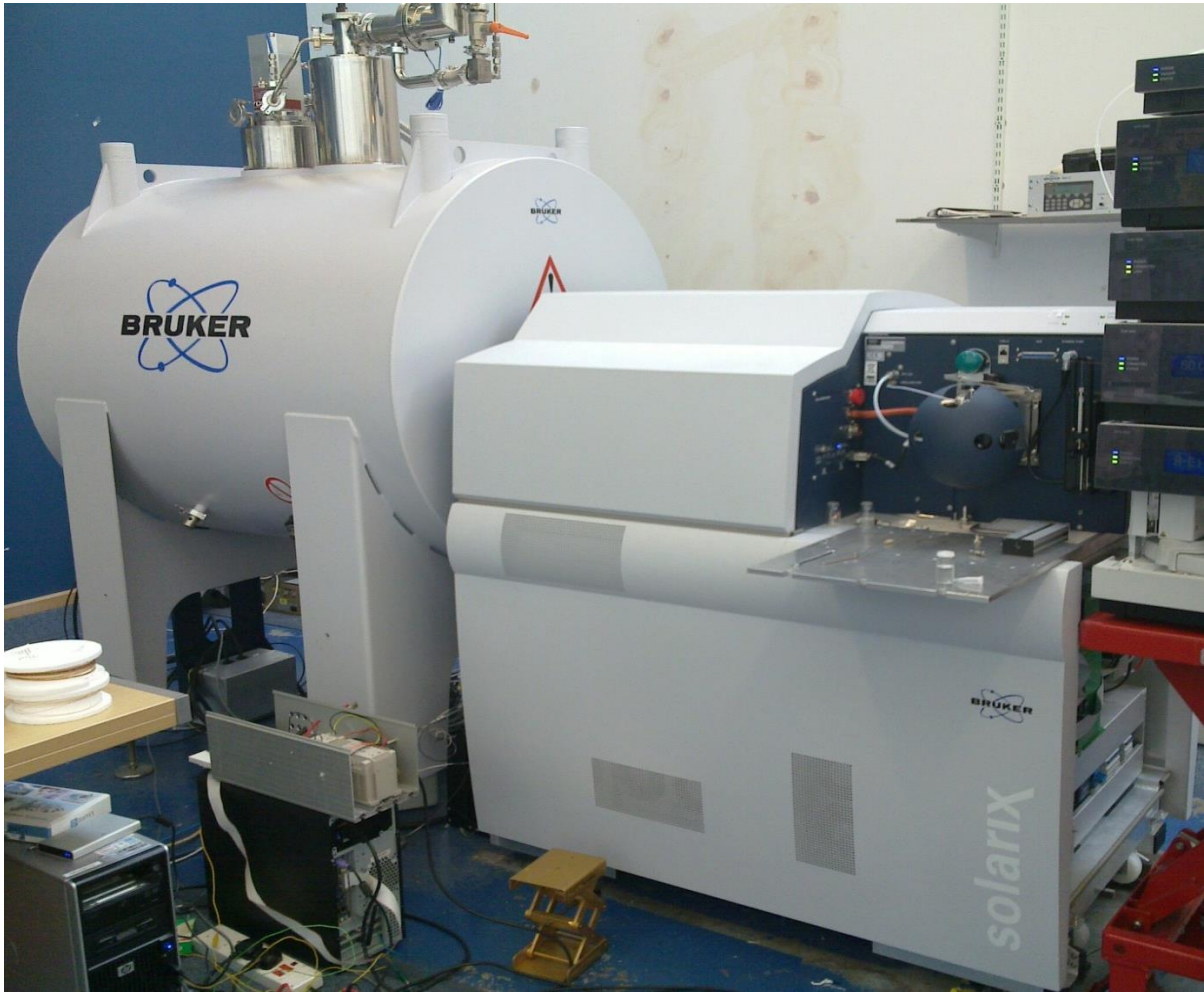
Figure 2.1: The Bruker solarix FT-ICR MS instrument coupled to a 12 Tesla superconducting magnet.
