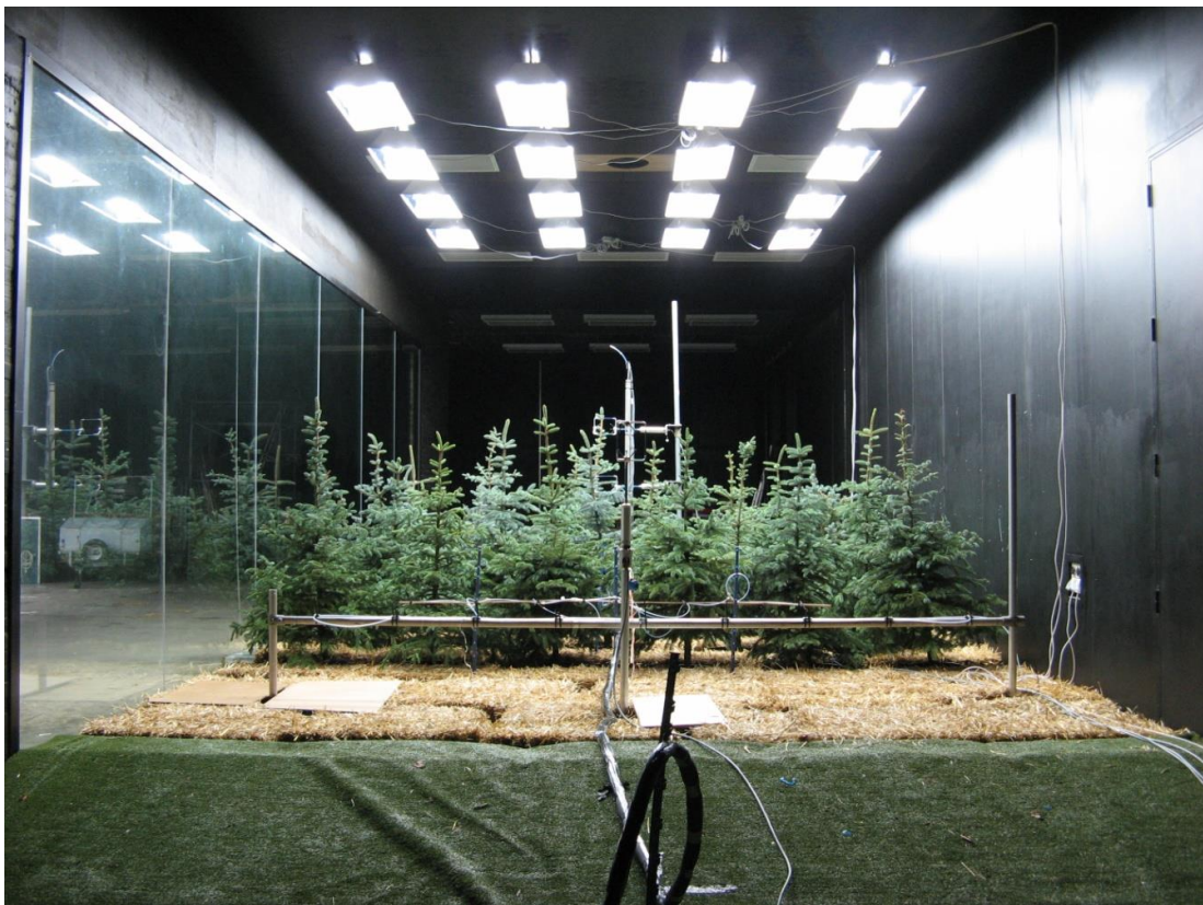
Figure 1.12: Side view of the wind tunnel with 28 trees and 16 growth lights on. (Bottom) Front view of the wind tunnel with 28 trees and 16 growth lights on.
