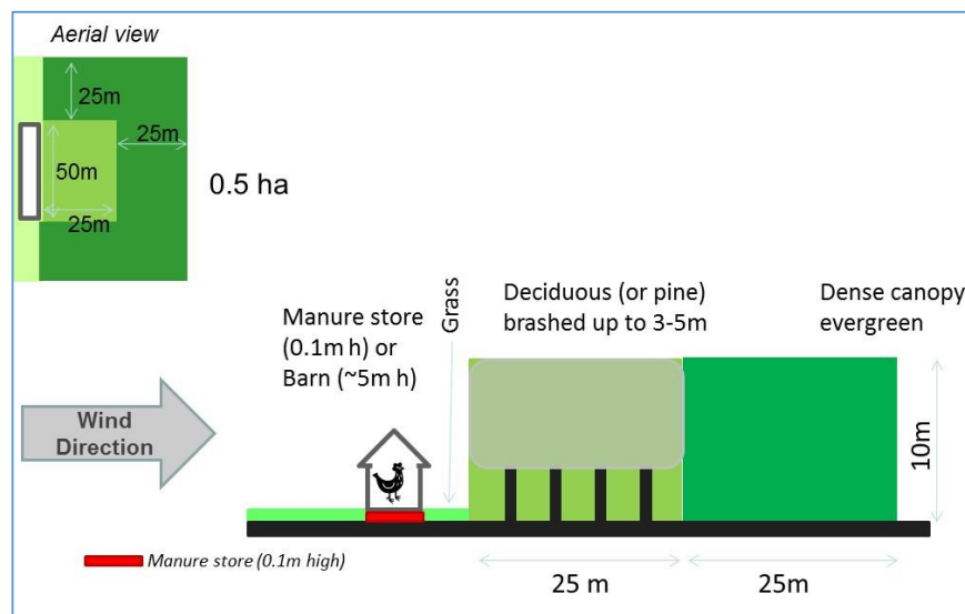
Figure 6.1. Schematic of Option 1: a tree planting design of 25 m depth of broadleaves trees with a Leaf Area Index (LAI) of 3, and a 25 m deep dense backstop with a LAI of 6. The aerial representation shows the dense 25 m backstop ‘wrapping’ around the main canopy. For a 50 metre long housing installation (shed) the overall tree design is 0.5 ha in size. The emissions come from the housing/manure store location.
