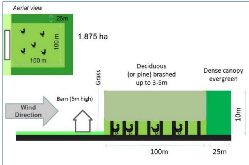
Figure 6.2. Schematic of Option 2: a tree planting design 100 m deep with broadleaf trees with a Leaf Area Index (LAI) of 3, and a 25 m deep dense backstop with a LAI of 6. The aerial representation shows the dense 25 m backstop ‘wrapping’ around the main canopy. For a 1 ha area of free ranging animals the overall tree design is 1.875 ha in size. The emissions come from the livestock under the canopy.
