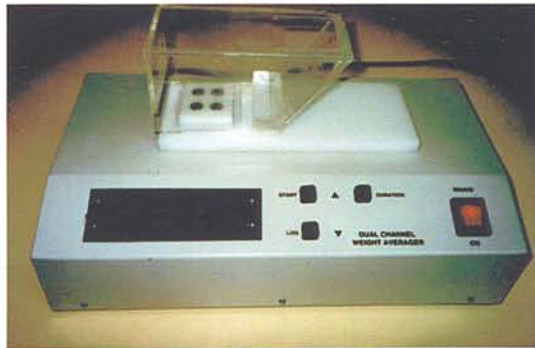
Figure 2.4 Photograph of the weight averager used to assess weight-bearing allodynia in monoarthritic rats.
