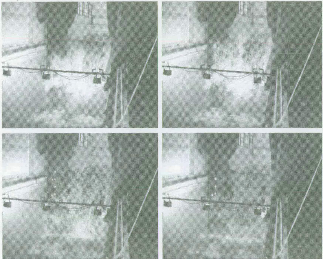
Figure 11: Synchronised video and throw detection at 0.17s intervals (Test series Big-VOWS C11 : H_s=0.67\text{m} , T_s=3.29\text{s} ).
