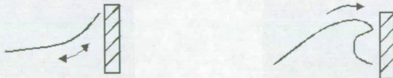
Figure 2: Pulsating (left) and impulsive (right) wave action at a wall.
