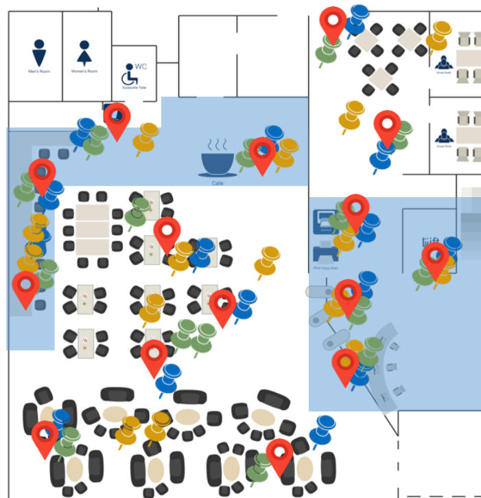
Figure 5.18 Test points estimation results of three methods on the ground floor. Red markers indicate the ground truth; yellow pins indicate magnetic field alone IPS; green and blue pins indicate Wi-Fi aided and camera aided segmentation strategy.
