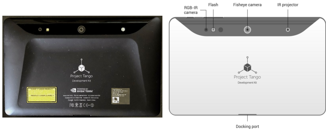
Figure 3.3 Example of Google project tango with the embedded sensors. A depth sensor embedded in RGB-IR camera is used to detect the distance to the target object and helped with building the 3D point cloud model of scanning environments [81].
