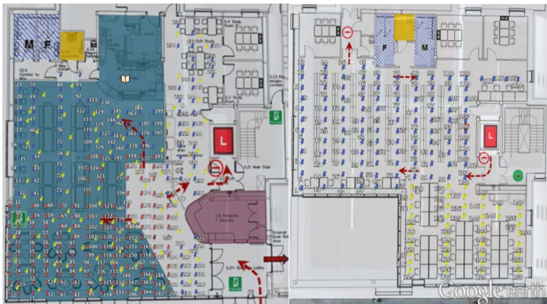
Figure 5.13 An illustration of sample points distribution on different indoor scenarios. 251 and 157 sample points were uniformly collected on the ground floor (left) and second floor (right) of KB library respectively.
