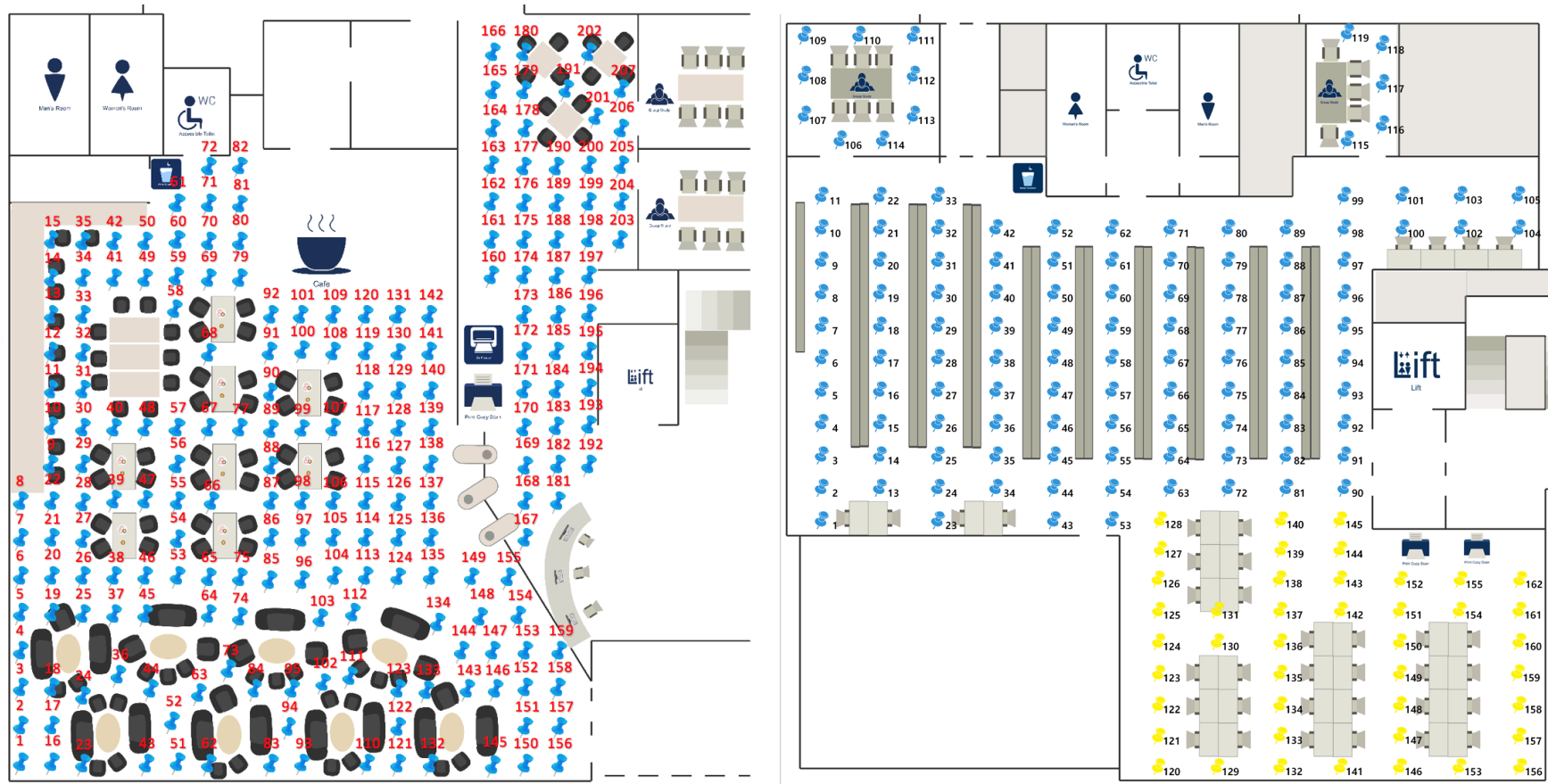
Figure 5.14 Distribution of sample points collected on the ground floor (left) and second floor (right). 207 and 162 magnetic sample points were collected and stored into floor fingerprint database.
