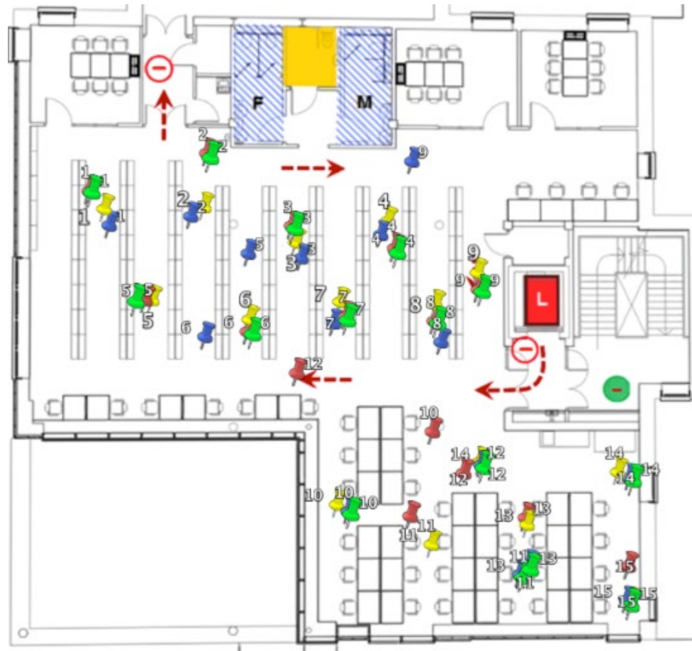
Figure 5.16 Test points estimation results of three methods on second floor. The yellow landmarks represent the locations of the ground truth, and the red, blue and green markers represent the estimated locations where the magnetic field-only, camera-only and offline segmentation strategy-based IPS were adopted respectively.
