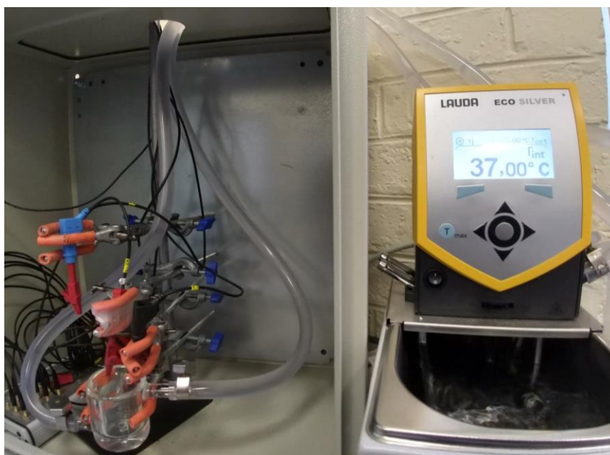
Figure 3-12: Photographs of the water-jacketed glass cell integrated with three-electrode system inside the Faraday cage and the thermostatic bath (Lauda Eco Silver) used for temperature-controlled experiments.
