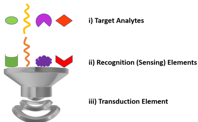
Figure 2-4: Schematic illustration of a chemical sensor, an assembled device consisting of two main components, a recognition and a transduction element in order to interact with a target analyte.
