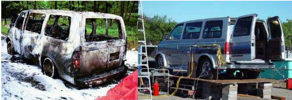
Figure 1. Vehicle testing site (right) and the post fire remains of the real case (left).
