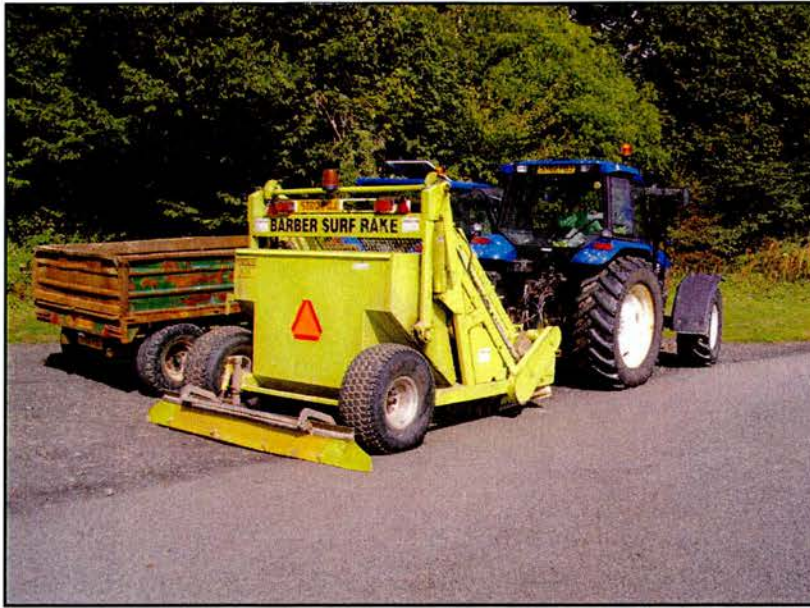
Figure 4.6: Mechanical Beach Cleaning Machine, Silversands 19/08/05
