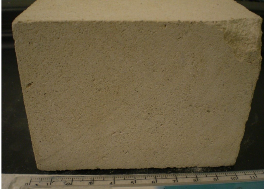
Figure 4-1: Photograph of Portland stone used in this study. The oolitic nature of the stone can be seen. The ruler provides a scale.
