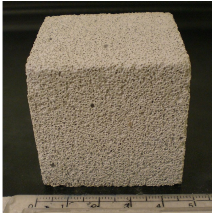
Figure 5-1: Photograph of an AAC sample prior to treatment. The macro pores of the material can be clearly seen. The ruler provides the scale.
