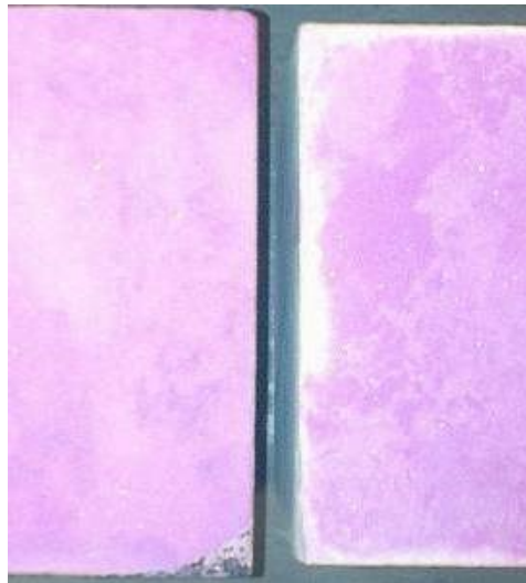
Figure 4-28: Phenolphthalein treated failure surfaces exposed by strength testing 25 minutes (left) and 25 hours (right) after adhesion. Pink areas, with higher pH, are uncarbonated.
