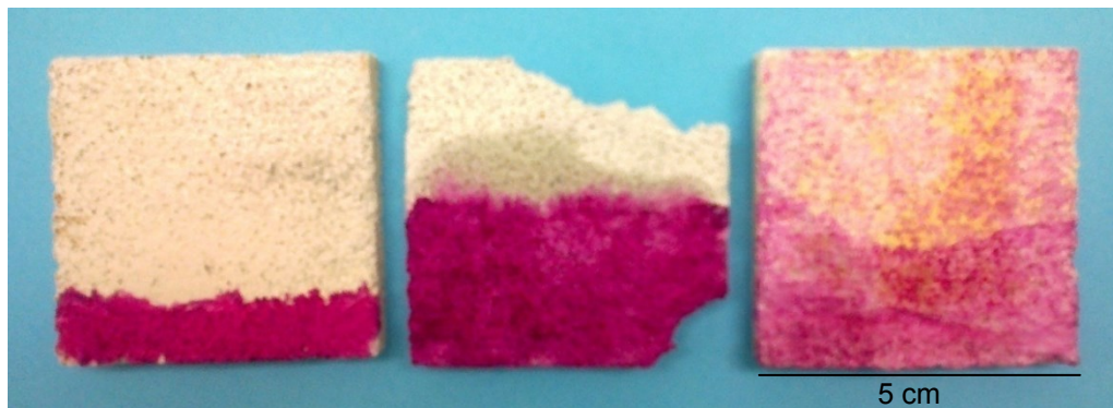
Figure 5-6: Photograph showing the internal height of treatment and extent of positive reaction with phenolphthalein indicator for (left to right) a thin layer sample, a medium layer sample and a thick layer sample. Scale bar is 5 cm.
