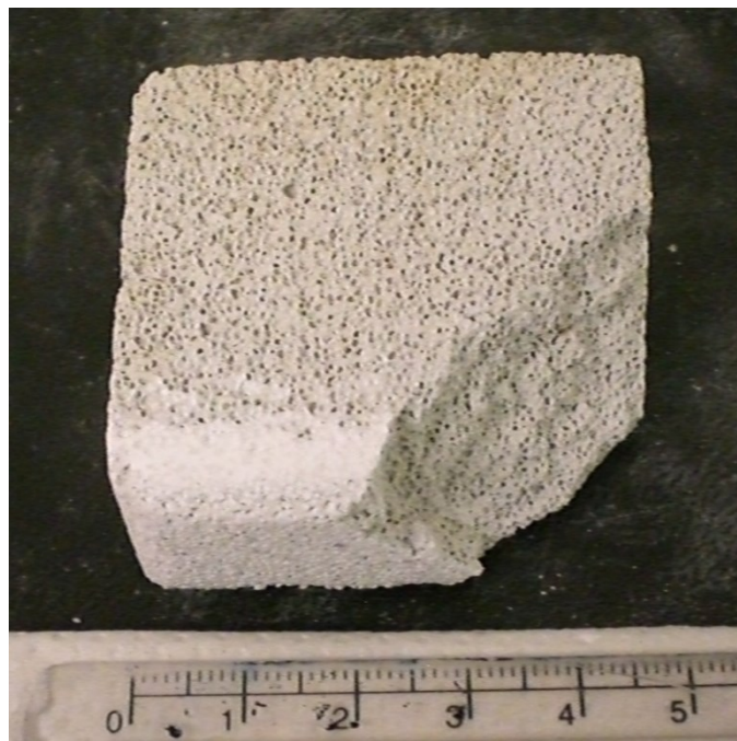
Figure 5-5: Photograph of a slice of an AAC sample treated to the thick layer (section of block missing was removed for investigation by optical microscopy). The treatment build-up on the surface of the sample can be clearly seen. The ruler provides the scale.
