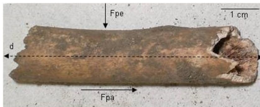
Figure 6-17: Diagram showing directionality of bone. d is direction of bone (long axis). Fpa is direction of force applied parallel to d. Fpe is direction of force applied perpendicular to d.
