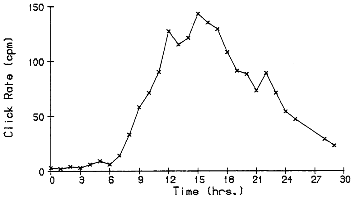
Figure 7.5. The time course for click production during a 30 hr. period of water loss in an excised apple stem (Arthur Turner).
