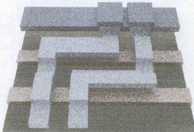
Figure 5.14: Conformal representation of layout 4 (figure 5.5), with interconnect track aspect ratios of one third.
