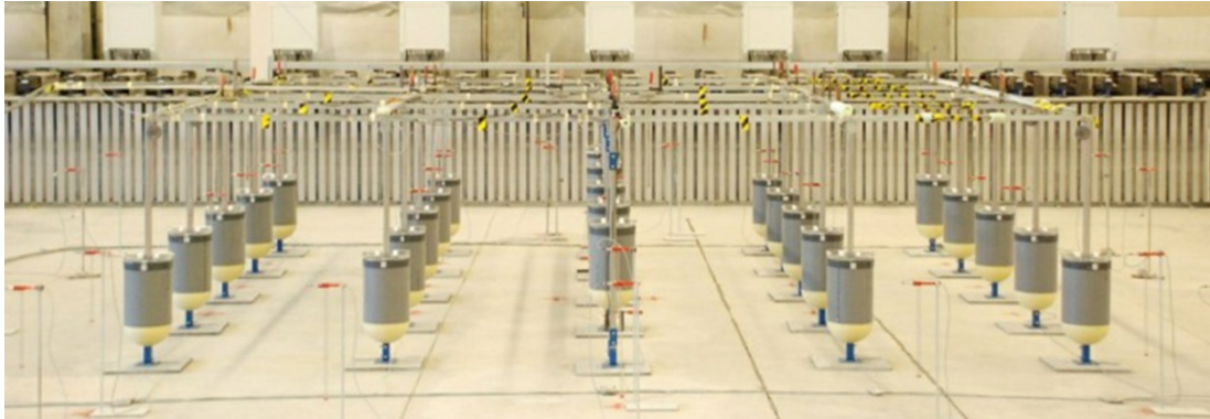
Figure 4.2: Photograph of the empty DHI shallow water basin containing the twenty five WECs and frame that form the experimental rig † .
