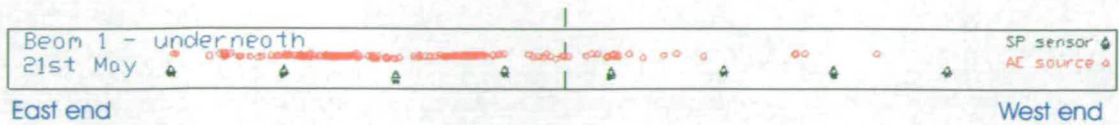
Figure 8.10: Boghall bridge. Location of the SP events, for Case 1. The green triangles represent the SP sensors, while the red circles show the located AE sources.
