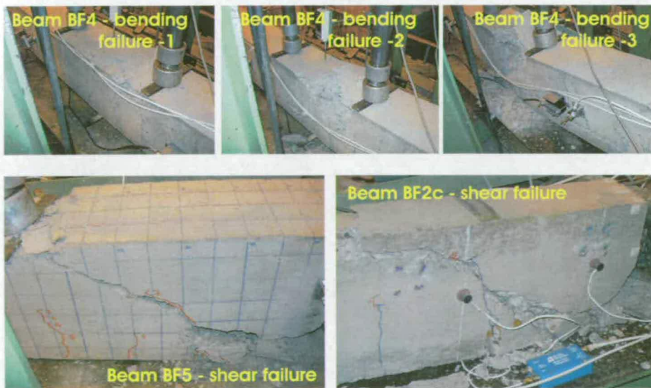
Figure 6.17: Photos of Edinburgh beam failures. Note the visible shear dislocation of the grid pattern for test BF5.
