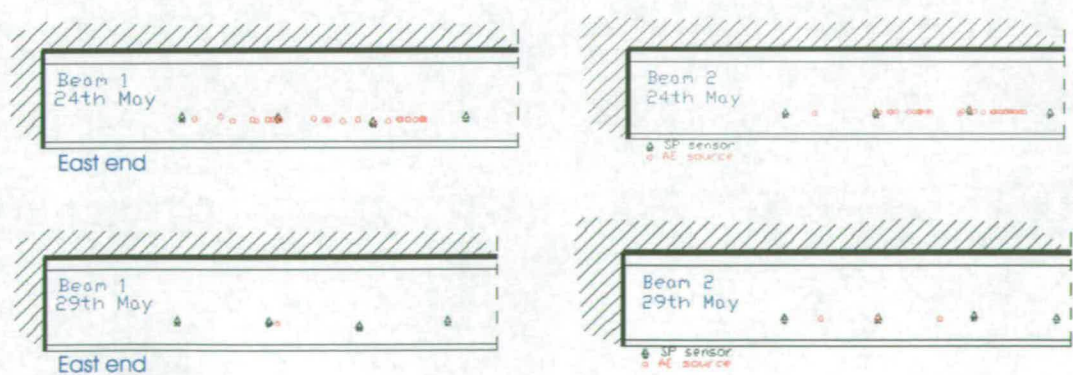
Figure 8.12: Boghall bridge. Location of the SP events, for Case 3, plotted as for Figure 8.10.
