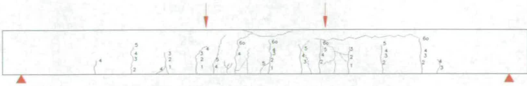
Figure 6.16: Final crack pattern of beam BF6.
