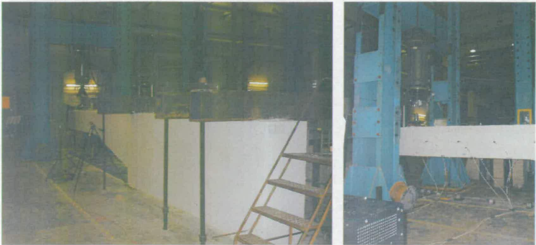
Figure 6.23: Beam HB2. Test configuration and instrumentation.
