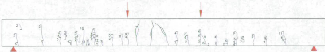
Figure 6.13: Final crack pattern of beam BF4.
