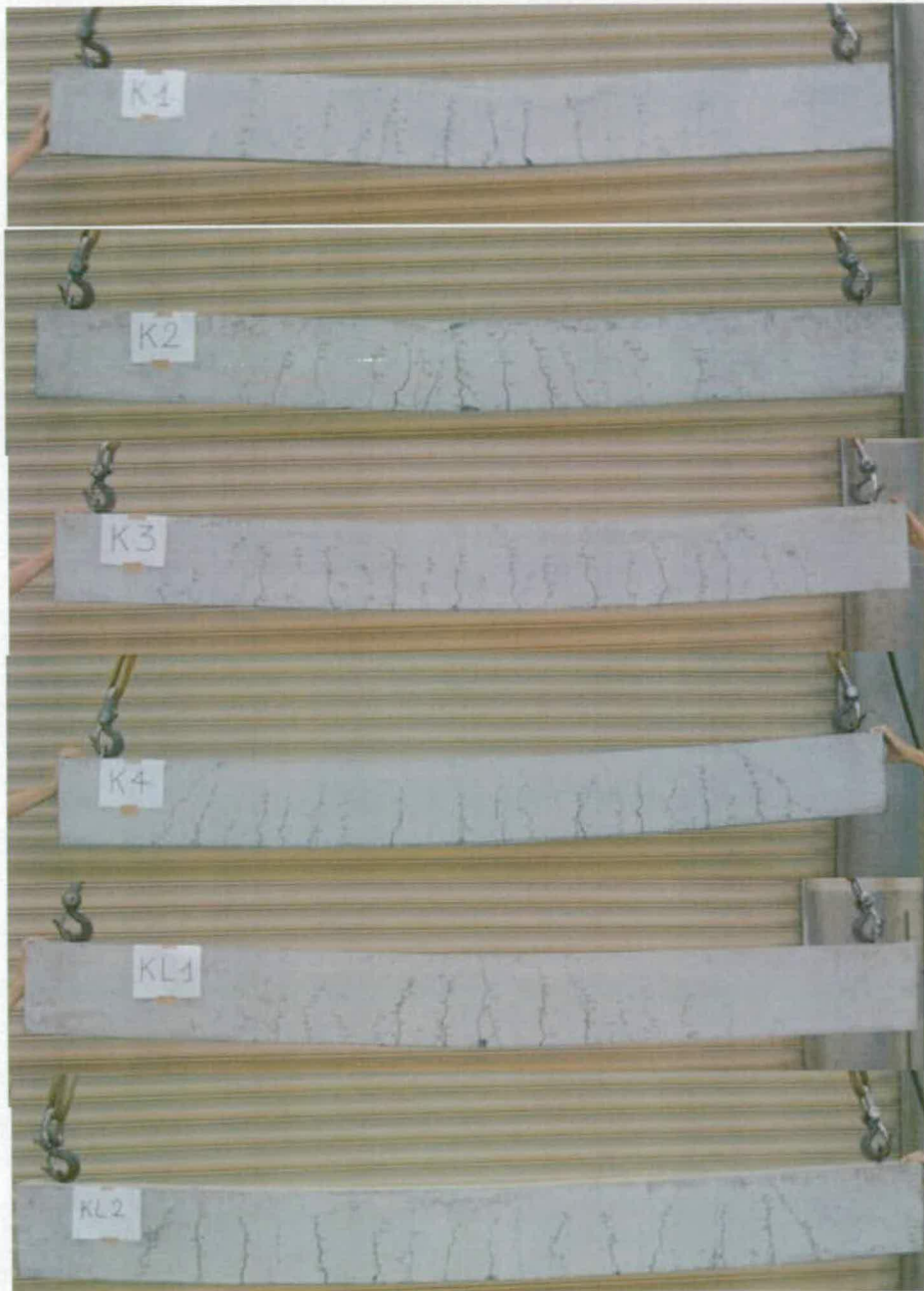
Figure 6.33: Photos of failed beams at Kumamoto Laboratory.
