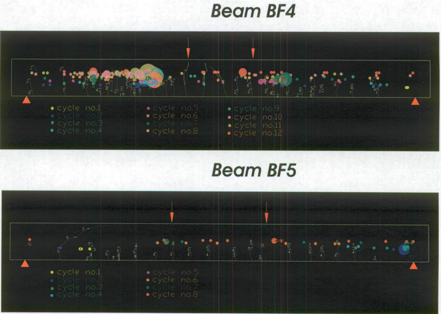
Figure 7.26: Location of events recorded by the SoundPrint system on beams BF4 and BF5. The different colors indicate different loading cycles, whilst the diameter is proportional to the number of events.
