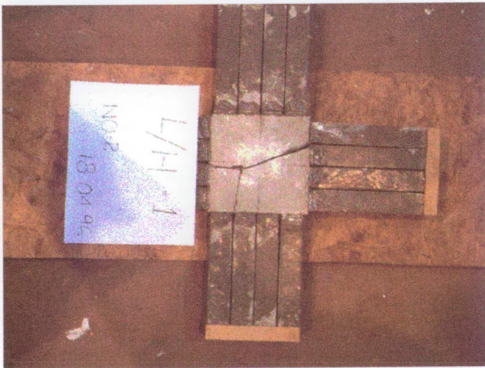
FIG. 4.14 Failure Pattern in Cross Beams (Aspect Ratio 1:0.75)
