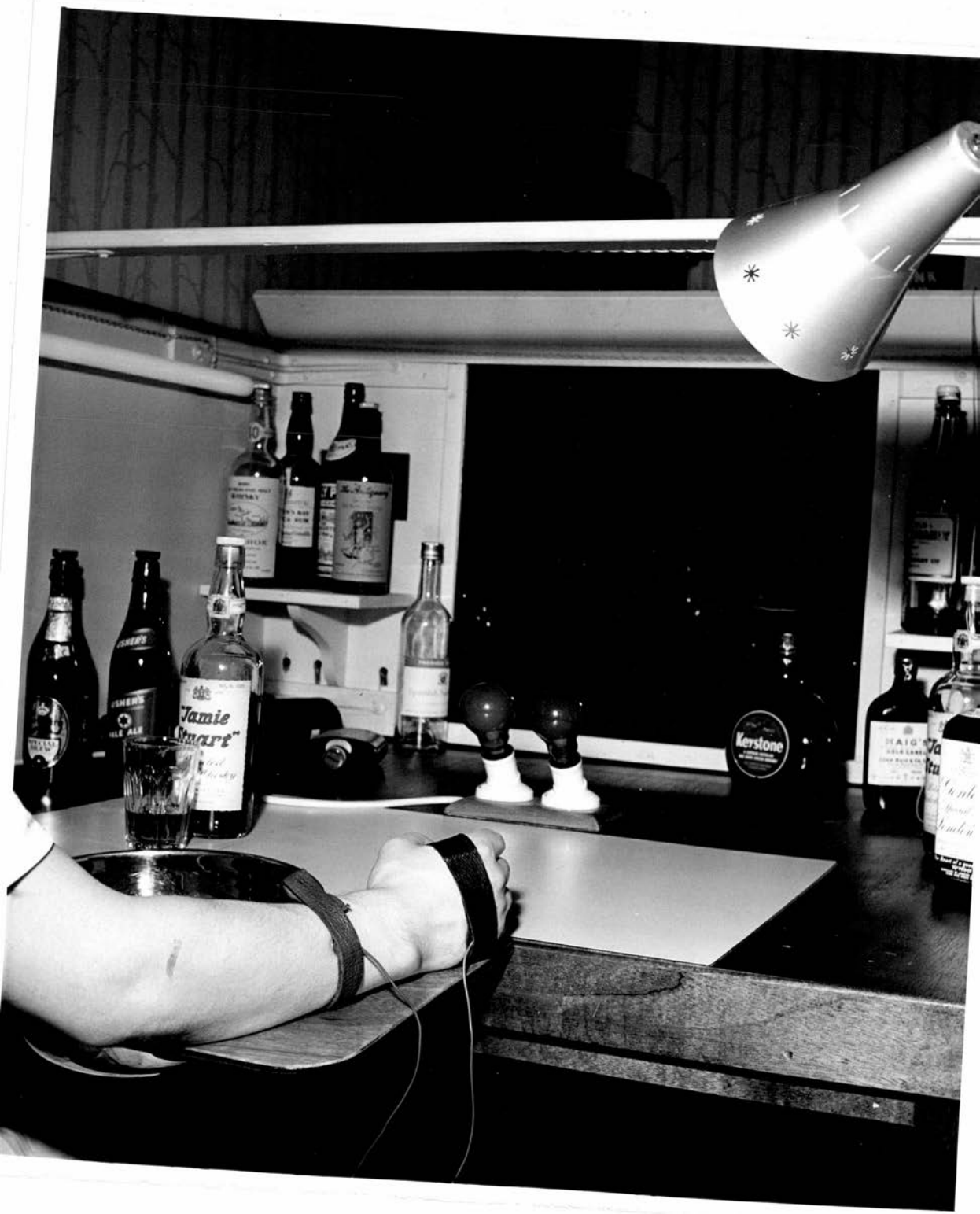
Plate 3. View of the Conditioning Cubicle from S's end: Illustrating position of Electrodes, and Red and Green Lights.
