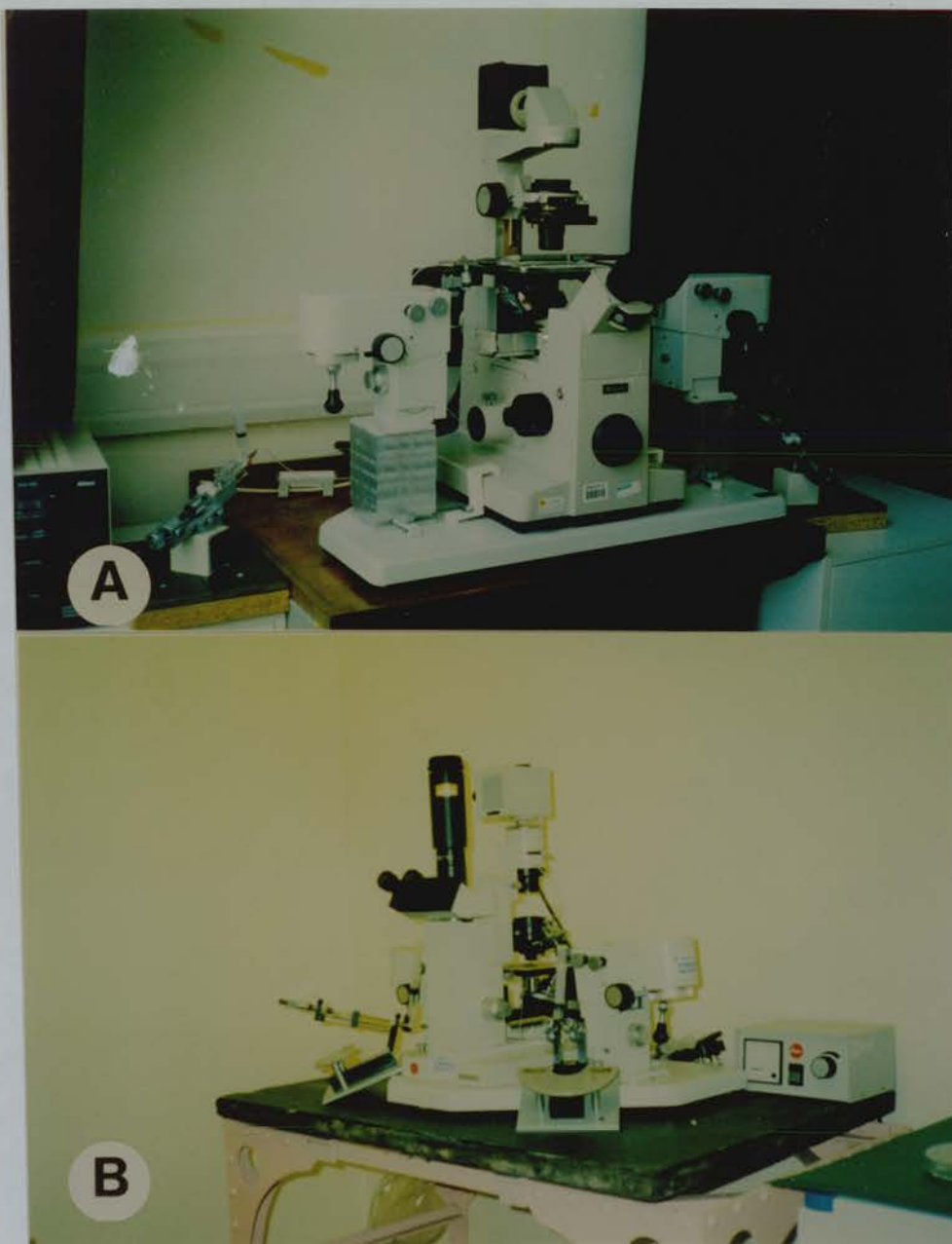
Fig. 4.2 The micromanipulation systems used in these experiments. A. The system used at Roslin Institute: a Nikon Diaphot TDM inverted microscope with Differential Interference Contrast (DIC) and epifluorescence, the Leitz M micromanipulators (manual model) associated with Narishige microinjectors (model IM-188) to hold two Hamilton (Sigma S-0142) syringes with a capacity of 500 \mu l, 250 \mu l for controlling the holding and enucleation pipettes respectively; B. The system used in the CRB: a Leitz Diavert microscope, the Leitz M micromanipulators (manual model) associated with RI microinjectors to hold one Hamilton syringe with a capacity of 100 \mu l for controlling the enucleation pipette and one 2 ml glass syringe (Weber Scientific) for controlling the holding pipette. All these manipulation syringes were connected to the tubes which go to the pipette holders with three-way taps that connect to another syringe containing fluorinert FC 77 (Sigma, F-4758; at Roslin Institute) or mineral oil (Sigma, M-8410; in the CRB) as a hydraulic reservoir.
