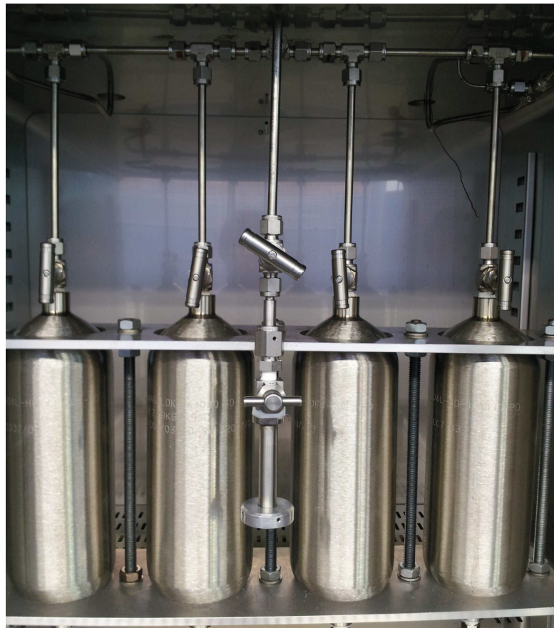
Figure 4.3: Capsule for the preparation of mixtures with liquids connected to the cylinders of the dosing oven.
