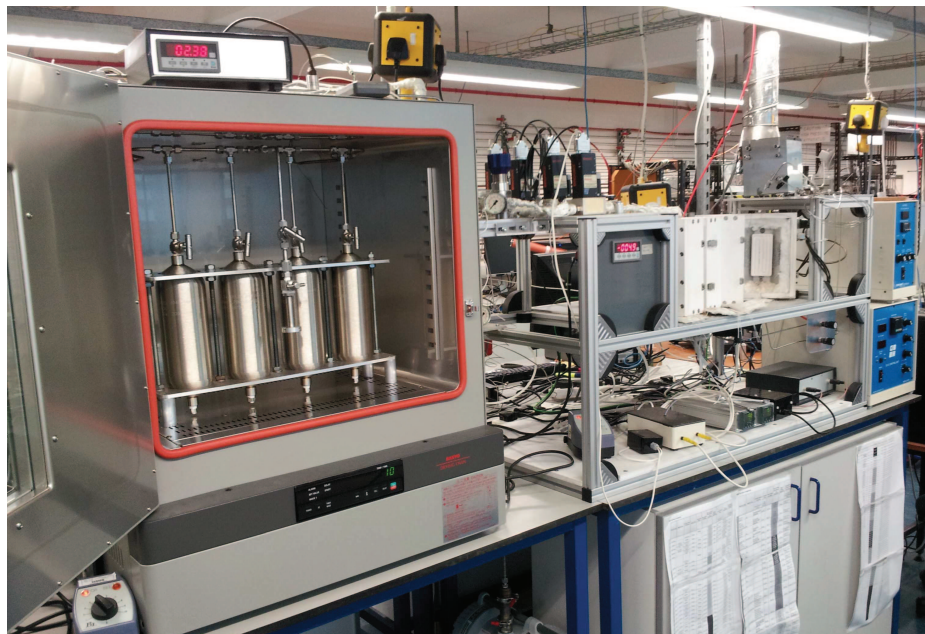
Figure 4.7: Semi-automated ZLC system.
