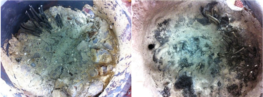
Figure 7-2: Representative comparison of concrete core colour and fragility for; (a) unprotected; and (b) protected CFS columns
