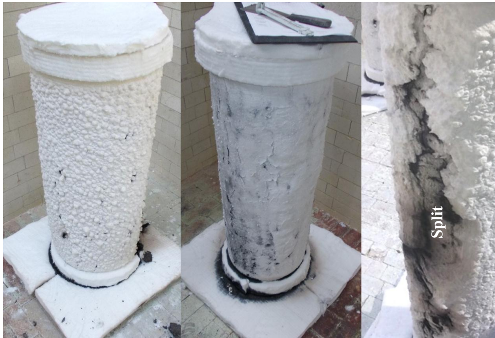
(a) (b) (c) Figure 5-21: Post burn intumescent coating reaction of (a) C11FIC1, (b) C11FIC2, and (c) C22FIC1 (split)
