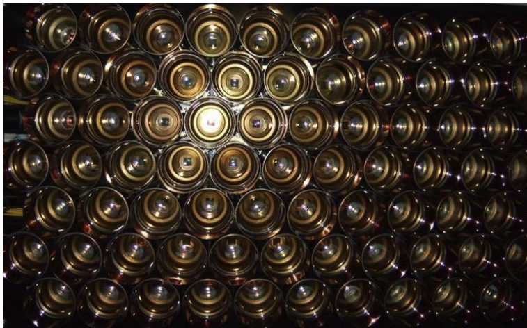
Figure 3.5: Photograph of the array of RICH 1 HPDs.
