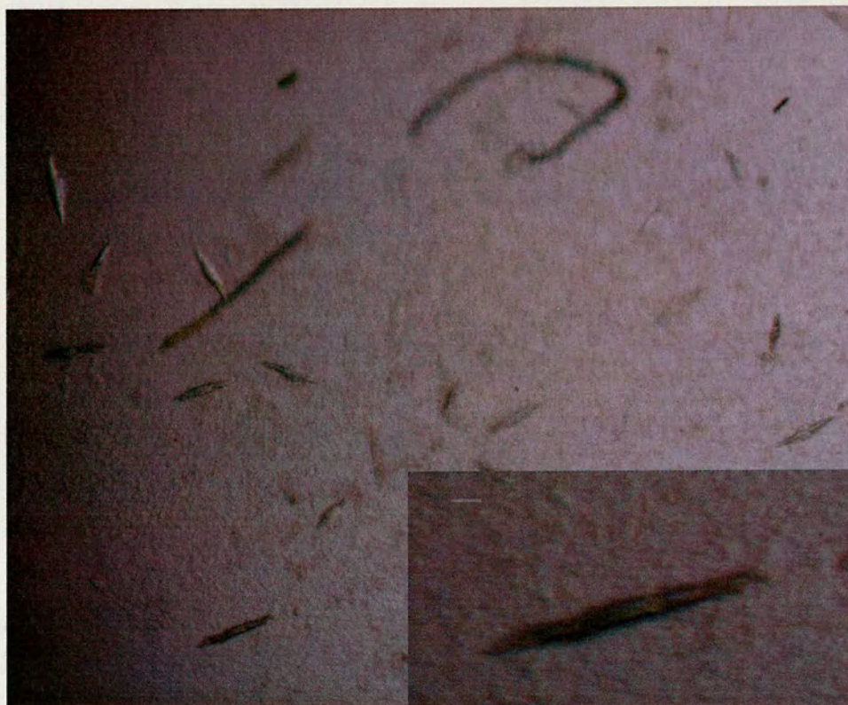
Figure 4.15. Crystals of hHsp90- \alpha 521. The crystals were tiny and formed a single needle-like shape (inset). The crystals were obtained from solution 4 of the Structure Screen 1 kit (MDL). Optimization experiments in an attempt to obtain better crystals were unsuccessful. The crystal did not diffract when screened on beamline 14.1 at CCLRC Daresbury.
