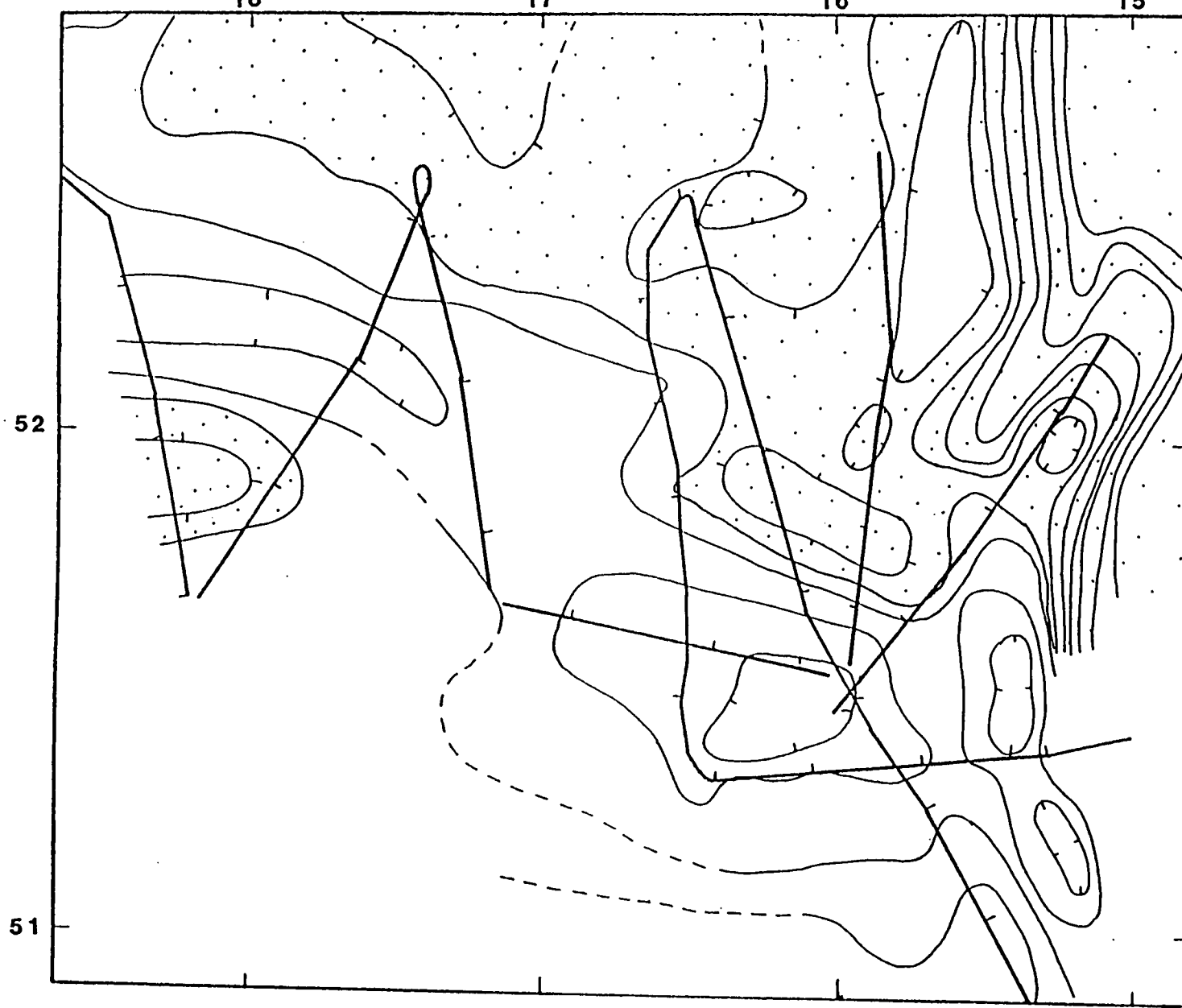
Fig. 5.4 Free air gravity anomaly map of the Clare Lineament - Charlie Gibbs Fracture Zone area. Contour interval 10 mgal. Stippled area : free air gravity anomaly >0 mgal
