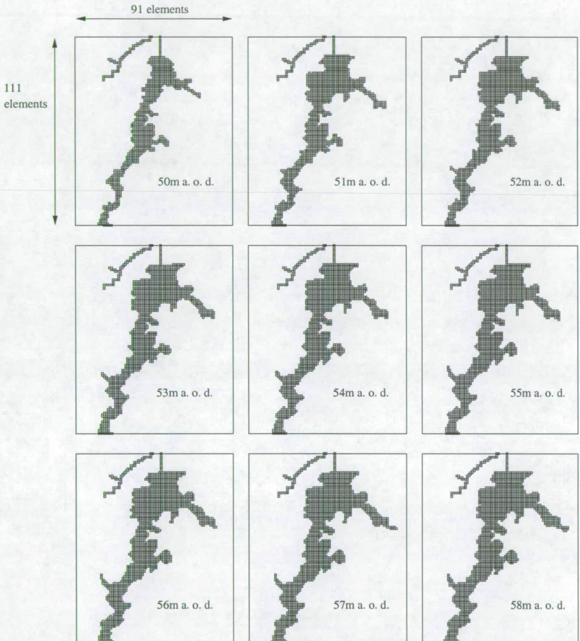
Figure 7.4: Figure showing the lake nodes for different lake levels. Here, some nodes were removed/added based on field data to correct some unrealistic effects of the interpolation and to add rivers Paraú and Açú (see text).
