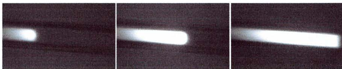
Figure 4-19 A series of video images showing an example of CE-LIF detection using rhodamine 6G. The capillary diameter is 50\ \mu\text{m} .
