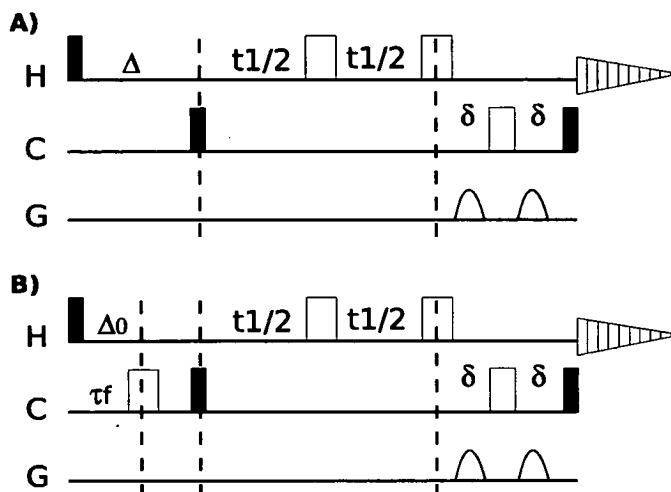
Figure 2.9: Pulse sequences of HMBC experiments used for multiplet reconstruction: Open and filled rectangles represent 180^\circ and 90^\circ pulses, respectively. The proton 180^\circ placed in the middle of the t_1 period refocuses proton chemical shifts. The final proton 180^\circ pulse ensures that the phase of HMBC multiplets is identical to the phase of left-shifted multiplets obtained from 1D TOCSY experiments. Figure A shows the pulse sequence used in conjunction with 1D templates. Figure B shows the pulse sequence with one-bond multiple-bond filter at the beginning of the sequence. This experiment also provides one-bond cross peaks that are used as templates.
