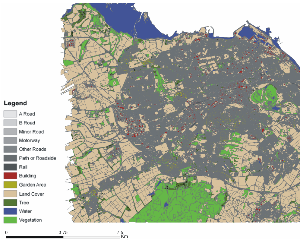
Figure 7.7: Source Database objects classified according to the pre-processing stage of the proposed methodology (Mapping is Ordnance Survey ©Crown Copyright. All rights reserved). The region is the city of Edinburgh and its surroundings in Scotland
