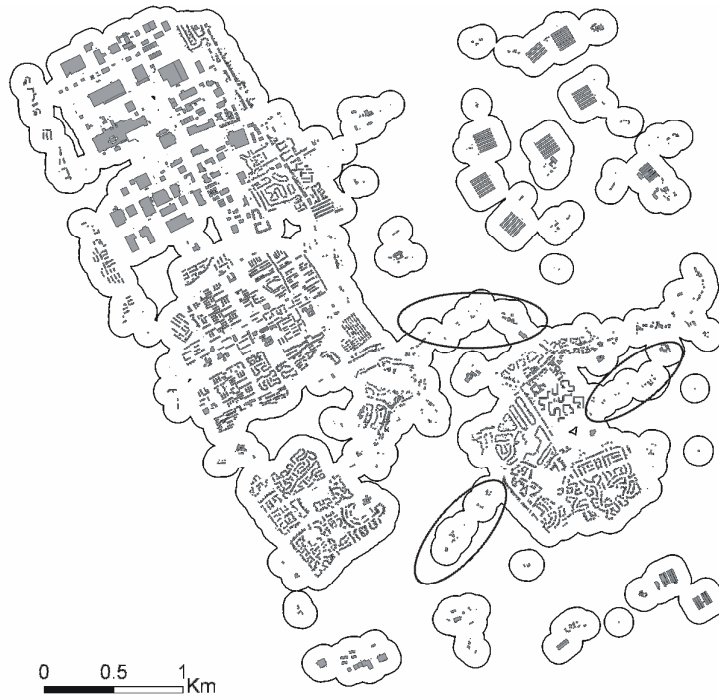
Figure 5.3: The output boundaries generated by distance based clustering algorithm using a 100m threshold. The low dense areas ringed in Figure 5.2 have become part of the output boundaries
