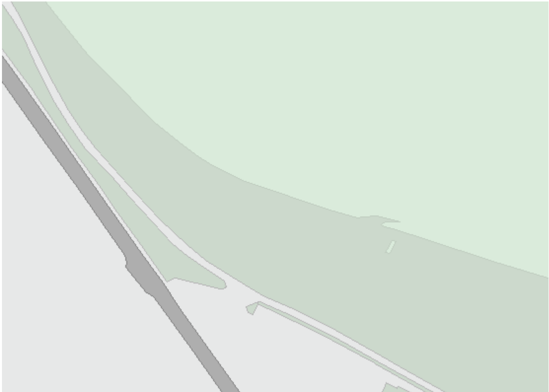
Figure 6.5: Overlapping composite objects due to m:n partonomic relationships for the region highlighted in Figure 6.2. The forest (light green) and settlement object (light grey) overlap because of aggregation based on multiple partonomies without any constraints
