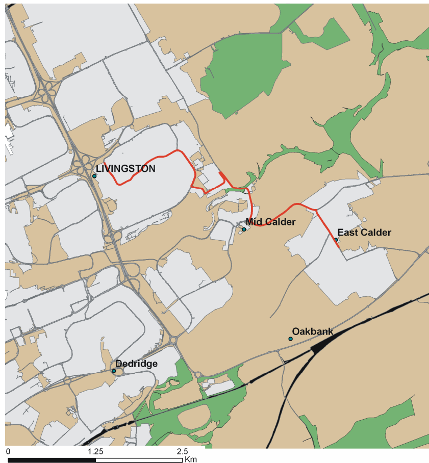
Figure 7.20: Example of spatial analysis. Finding the shortest road path (highlighted in red) between 'Livingston' and 'East Calder'
