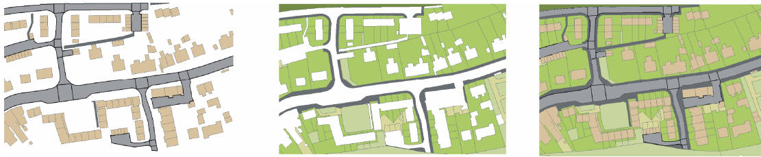
Figure 4.2: Polygon features form a complete geometric partition i.e. there is no overlap between features
