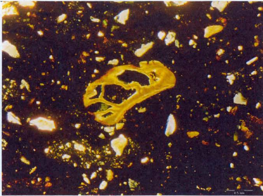
Plate 9: As Plate 8, but in XPL. Burned fragment appears birefringent.
