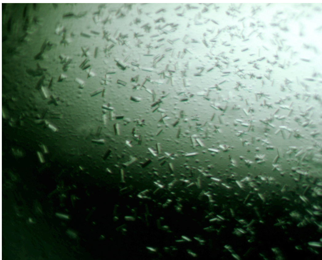
Figure 4.8 – Grown in 100 mM sodium acetate, pH 4.6, 2 M sodium formate (A4). The crystals appear to be small, nucleated needles that were indicative of crystals grown in the other conditions tested. Each crystal is roughly 10-20 \mu\text{m} long.
