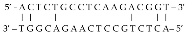
Figure 4.24 – A diagram showing the areas where the template strand could dimerise with itself
