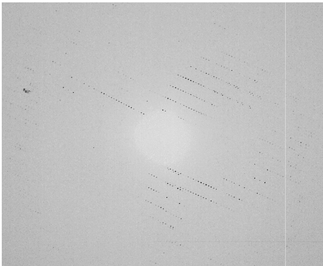
Figure 4.37 - Typical example of collected data during the high-pressure experiments. This particular image is from the 7th crystal shot during the experiment. The resolution limit was approximately 3.5 Å.
