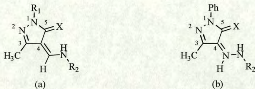
Figure 4.1. (a) 1-substituted-3-methyl-4-(alkylaldenamine)-pyrazol-5-thiones where \text{X} = \text{S} and pyrazol-5-ones where \text{X} = \text{O} and \text{R}_1, \text{R}_2 = a range of alkyl and aromatic groups, (b) 1-phenyl-3-methyl-4-phenylhydrazono-pyrazol-5-thione(ones).
