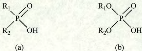
Figure 1.18. Weak extractants based on (a) phosphinic and (b) phosphoric acids.
