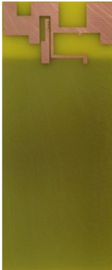
Figure 4.14 Fabricated prototype of the proposed dual-band PIFA
