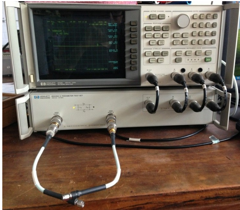
Figure 4.15 HP8753C vector network analyser
