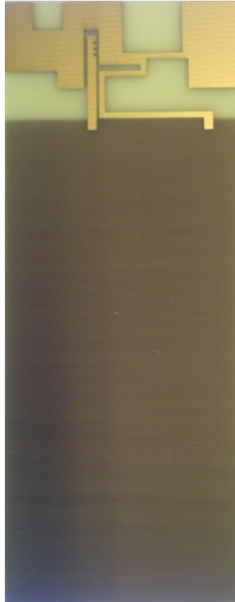
Figure 4.27 Fabricated prototype of the proposed triple-band PIFA
