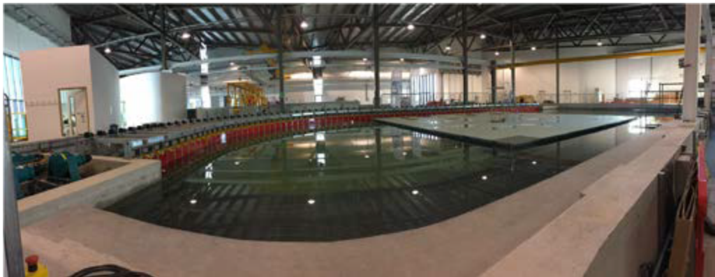
Figure 5.2.2.: Wave basin picture showing the movable floor in a raised position at Lir NOTF.
