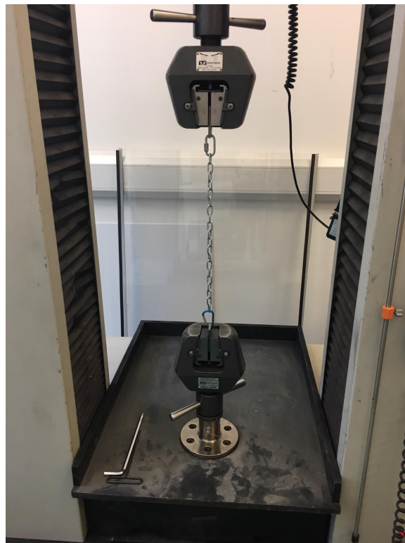
Figure 5.8.2.: Catenary axial stiffness experiment as performed in the structural laboratory.
