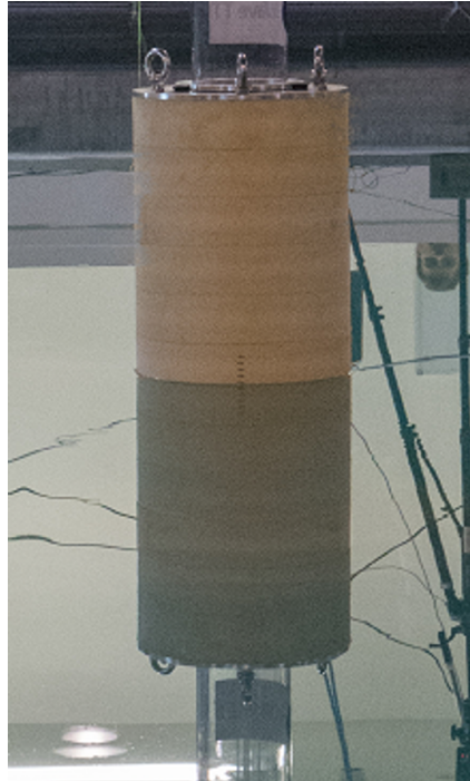
(a) Draft of the floater without mooring lines.
