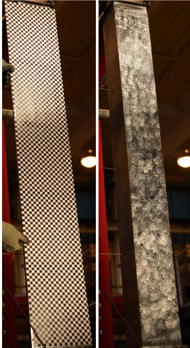
Figure 3.11: Checkered board used for DIC correction
