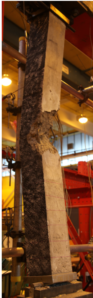
Figure 4.16: Typical mode of reinforced concrete columns in heating and cooling
