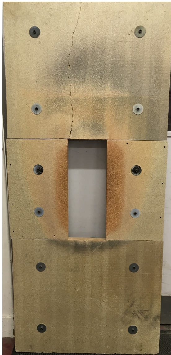
Figure 3.15: Shield used to expose only a defined area to the incident radiant heat flux induced by the radiant panels
