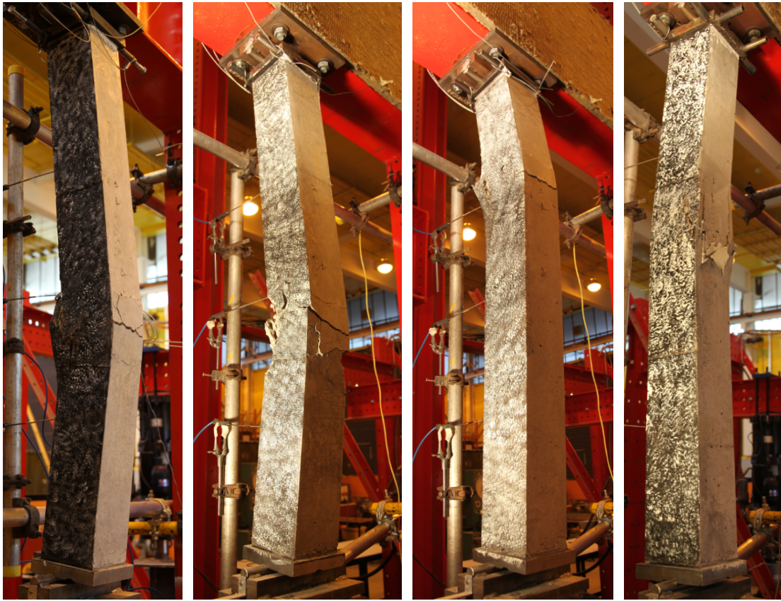
Figure 4.2: Typical failure mechanisms of reinforced concrete columns
