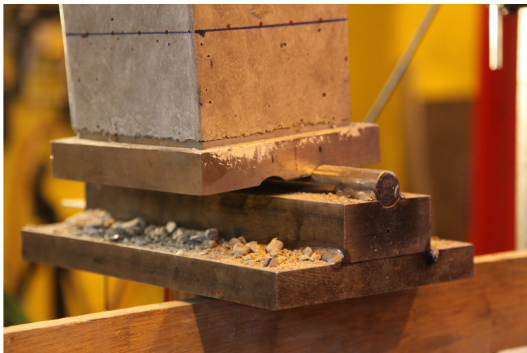
Figure 3.14: Interface between the loading plates and the steel caps attached to the columns
