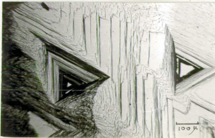
Typical 'growth' run etching of GaAs III A face showing characteristic triangular pits and steps
