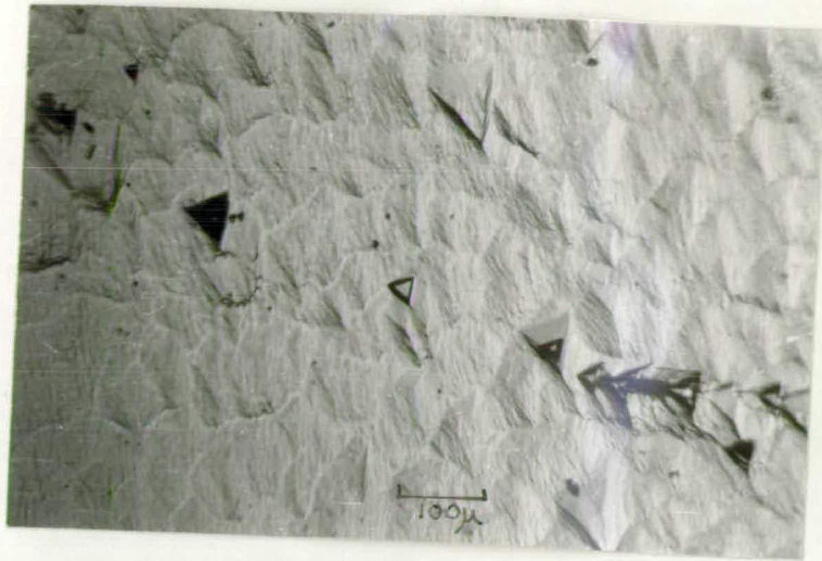
Hydrogen thermal etching x100
