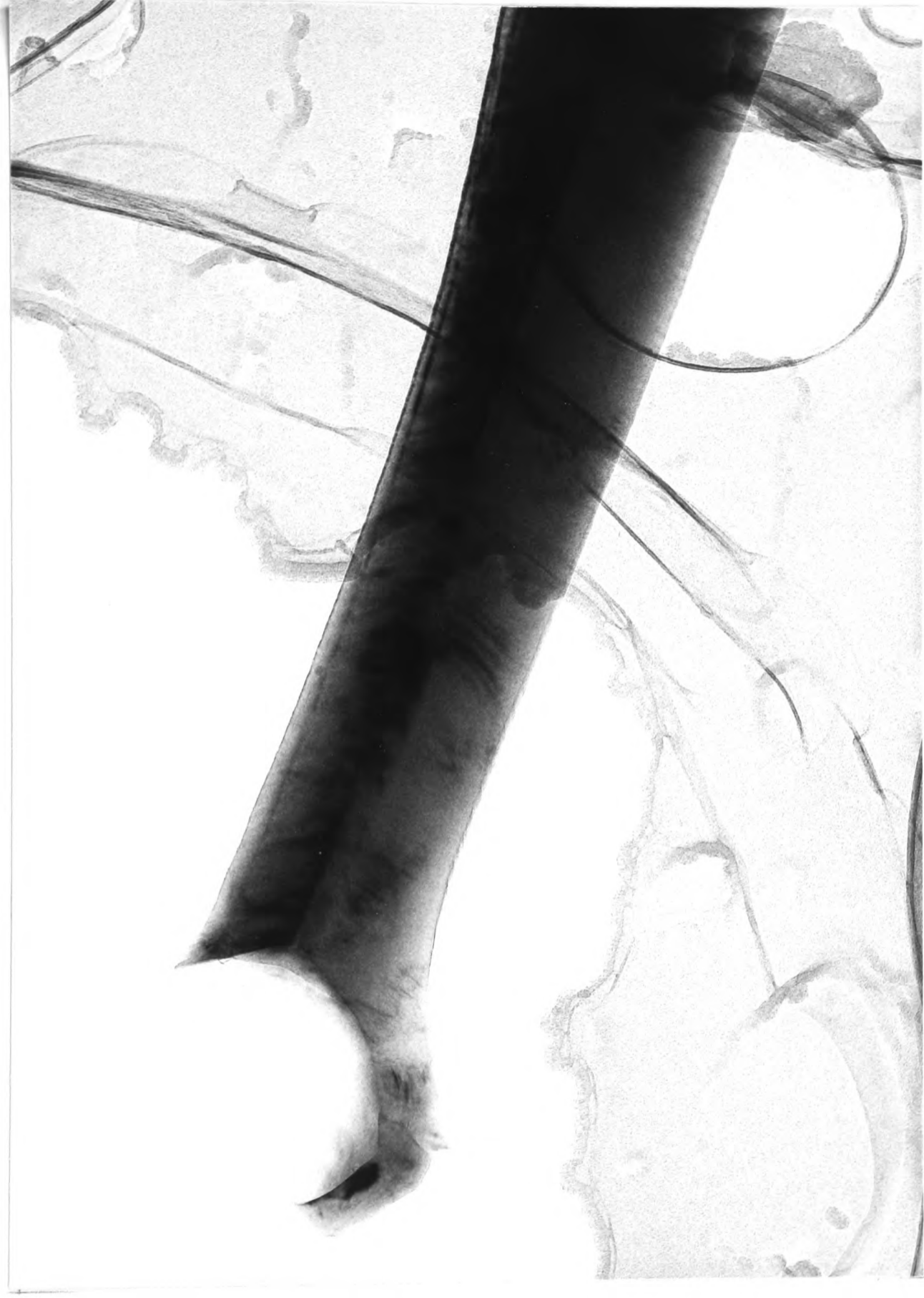
FIG. 6.2 - 20 : HREM OF NEEDLE SHOWING CONCAVITY
