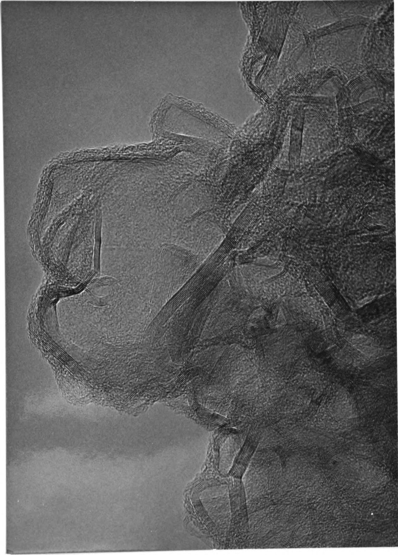
FIG. 6.2 - 4(c): HREM OF OXIDIZED PGC 69
