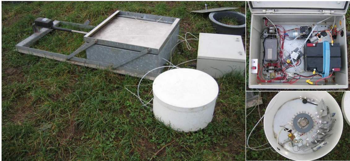
Figure 2.3: Automated gas flux sampler with external sampling box showing the Cali-5 Bond foil bags (bottom right) and power control unit (top right), (Chapter 3).
