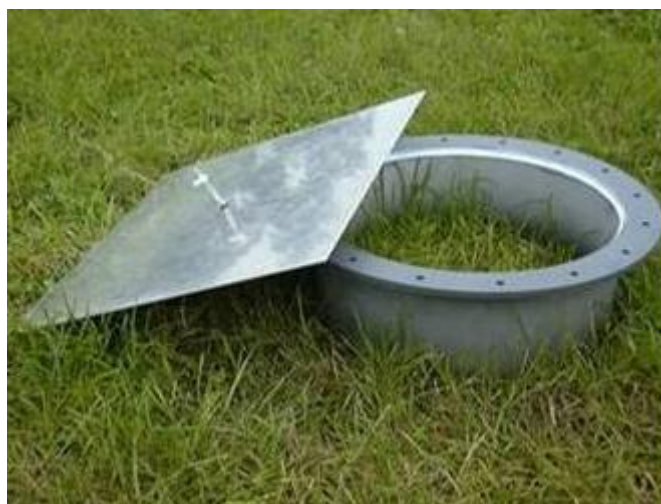
Figure 2.2: Static chamber design used for weekly flux measurements, (Chapter 3)
