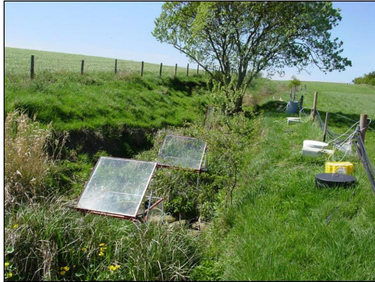
Figure 5.2: View of the constructed instream wetland in May 2007 from approximately 18 m along the water sampling transect which starts beneath the tree. Two of the transparent automated gas flux chambers in the wetland and control and sample boxes along the bank are apparent.
