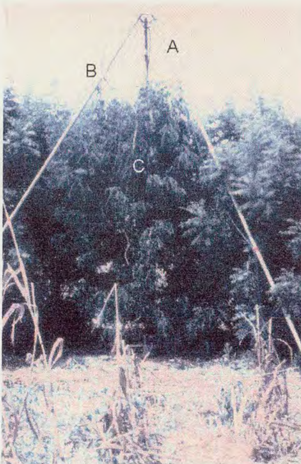
Figure 4.4: An Azadirachta indica tree (C) in a windbreak at Sadoré suspended from a load cell hanging from the apex of a tripod constructed from steel pipe (A). Nozzles (B) mounted on the legs of the tripod were used to spray water onto the tree and reference meteorological data were measured with a psychrometer, anemometer and wind vane mounted adjacent to the windbreak (not shown).
