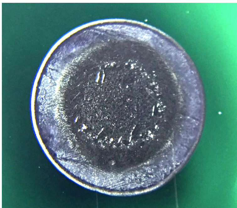
Figure 4.17: Image of a carbon microparticle OCPC in its dried state. During polymerisation the carbon has migrated into the centre of the droplet, leading to a black carbon rich region surrounded by a clear region of pure polymer. The carbon loading was 20 mg/ml. The cross-link density was 0.6 mol% wrt monomer MBA, 0.4 mol% wrt monomer oligonucleotide cross-linker.
