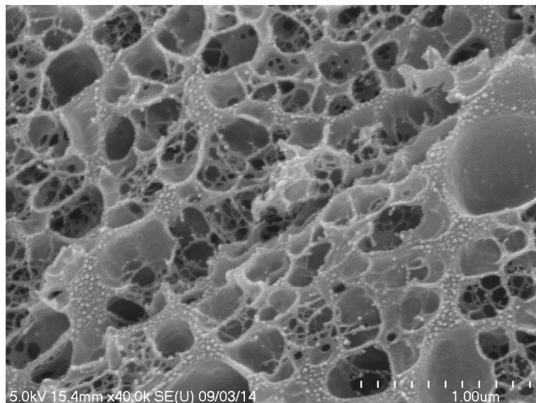
Figure 3.8: CryoSEM image of polyacrylamide/carbon nanopowder composite. The carbon loading was 5 mg/ml. The cross-link density was 0.6 mol% wrt monomer MBA, 0 mol% wrt monomer oligonucleotide cross-linker.
