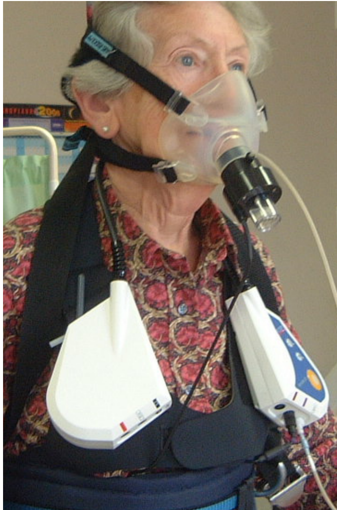
Figure 7.1 Metamax 3B metabolic measurement system as worn by a participant. The facemask houses a turbine to determine minute ventilation and a sample tube through which respired gases are continuously drawn. The system on the chest analyses performs breath-by-breath respiratory gas analysis, including calculation of \dot{V}O_2 . These data can be viewed in real-time on a remote computer via telemetry.
