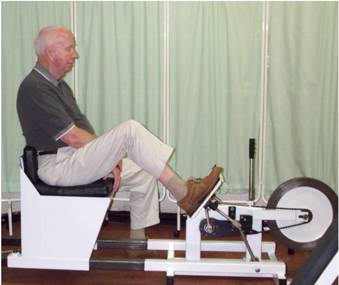
Figure 8.1 Healthy volunteer in the ‘start position’ prior to having the explosive power output of their right leg measured using the Nottingham Power Rig.
